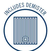
This product includes a mirror and Thermomirror demister. These are supplied as separate parts and the demister will need to be adhered to the back of the mirror prior to installation of the mirror. For details on the demister, please see next page
