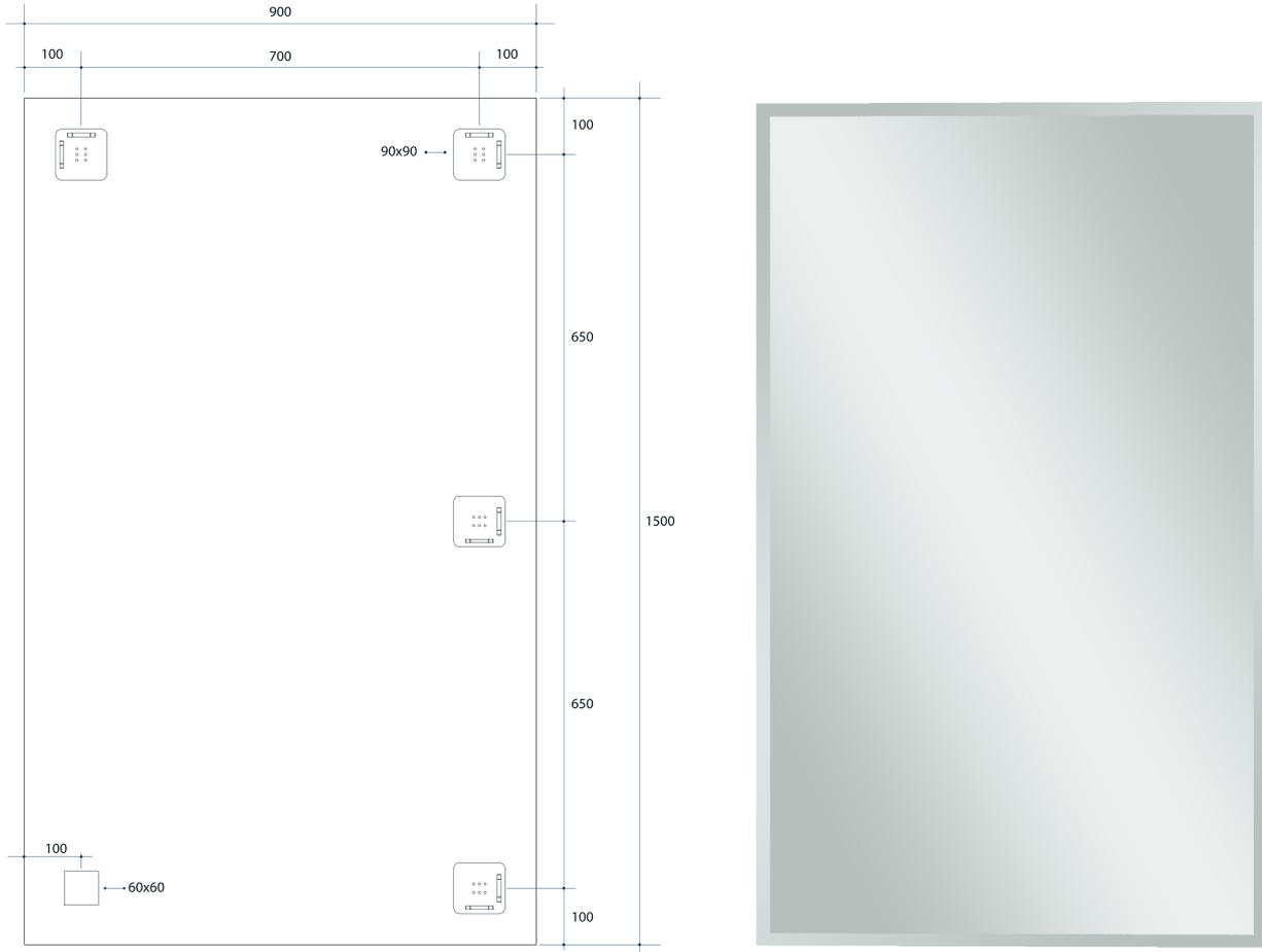
Note: All dimensions are in millimetres (mm)
